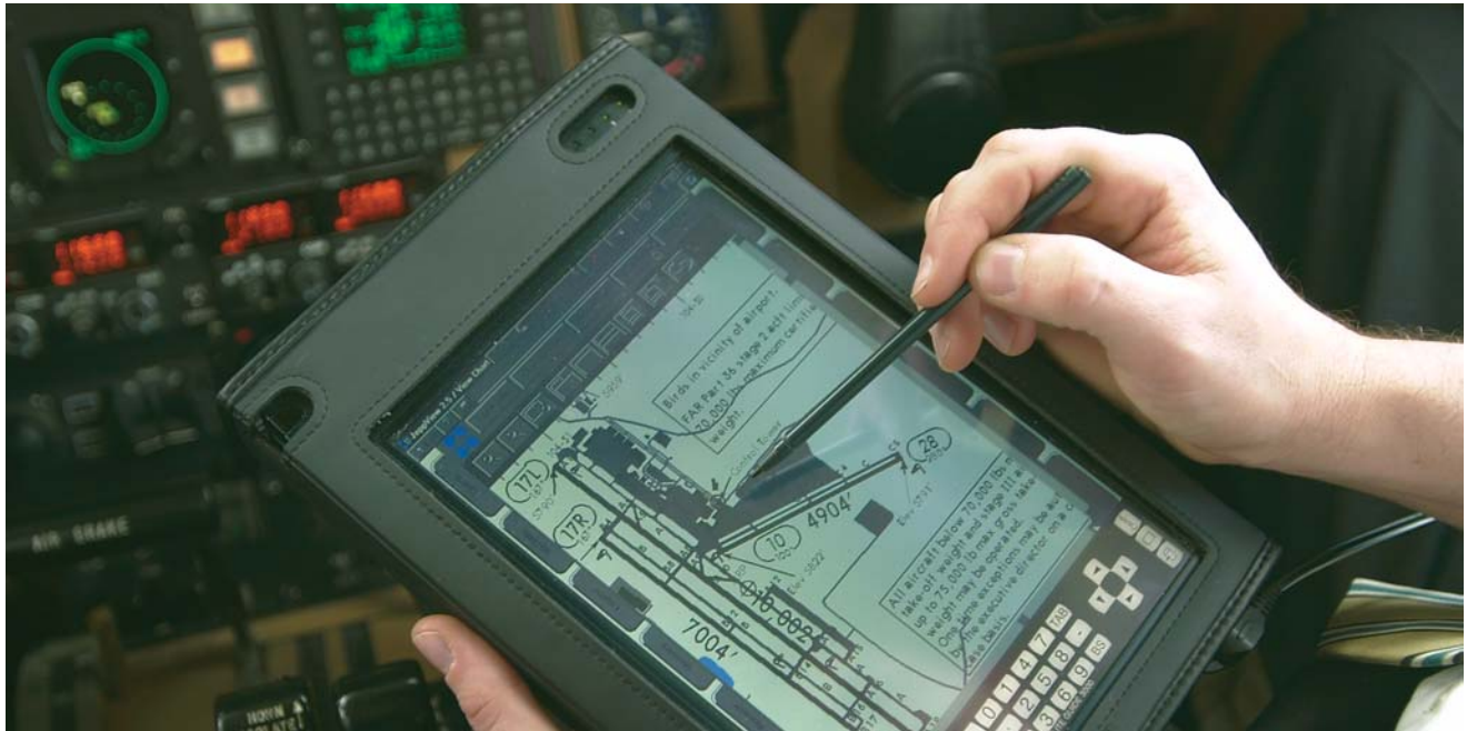
Figure 6-4. Electronic Flight Bag. The EFB has the potential to replace many paper charts and manuals in the cockpit.
