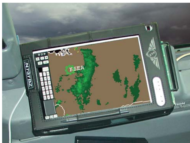
Figure 6-12. Prototype Data Link Equipment. This display shows a radar image of weather within 50 NM of the Seattle-Tacoma International Airport (KSEA).
