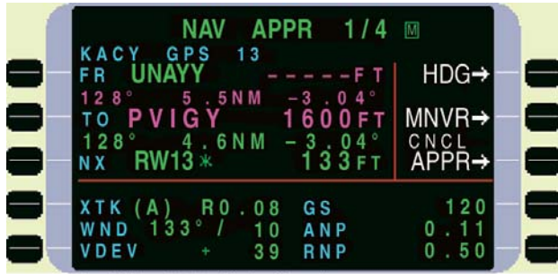
Figure 1-14. FMS Control Display Unit. This depicts an aircraft established on the Atlantic City, NJ, RNAV (GPS) Rwy 13 instrument approach procedure at the Atlantic City International Airport, KACY. The aircraft is positioned at the intermediate fix UNAYY inbound on the 128 degree magnetic course, 5.5 nautical miles from PBIGY, the final approach fix.
