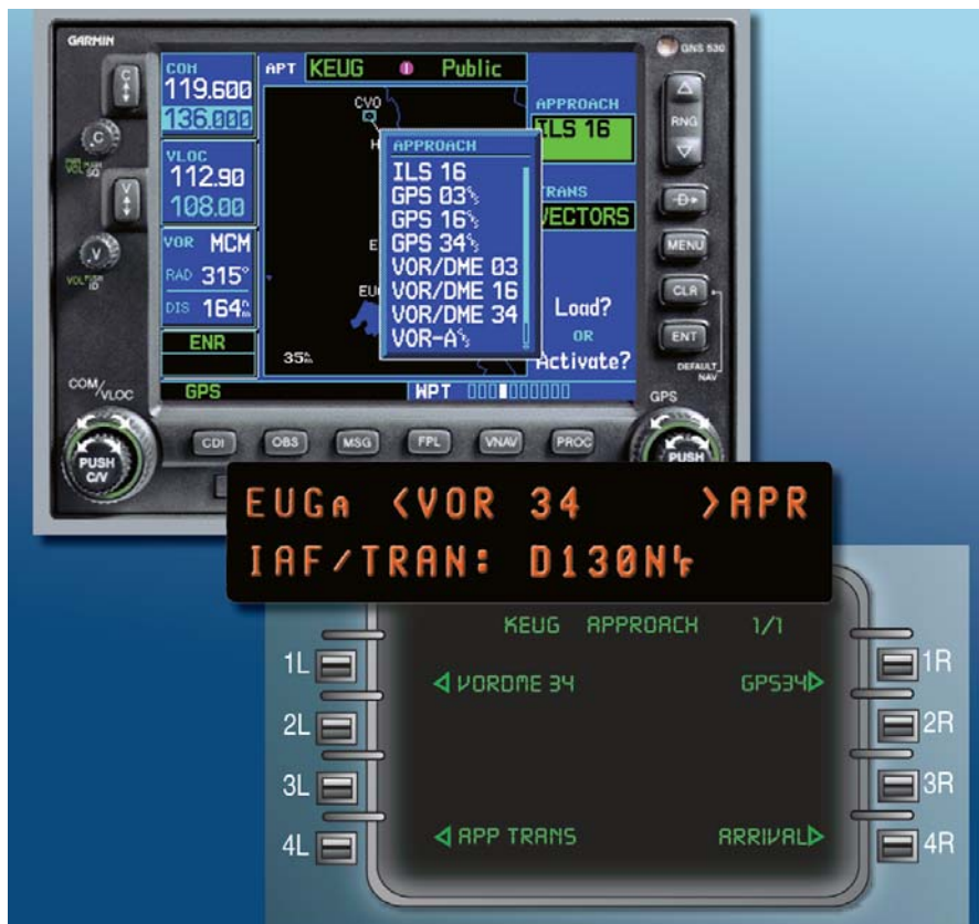
Figure A-2. Naming Conventions of Three Different Systems for the VOR 34 Approach.
