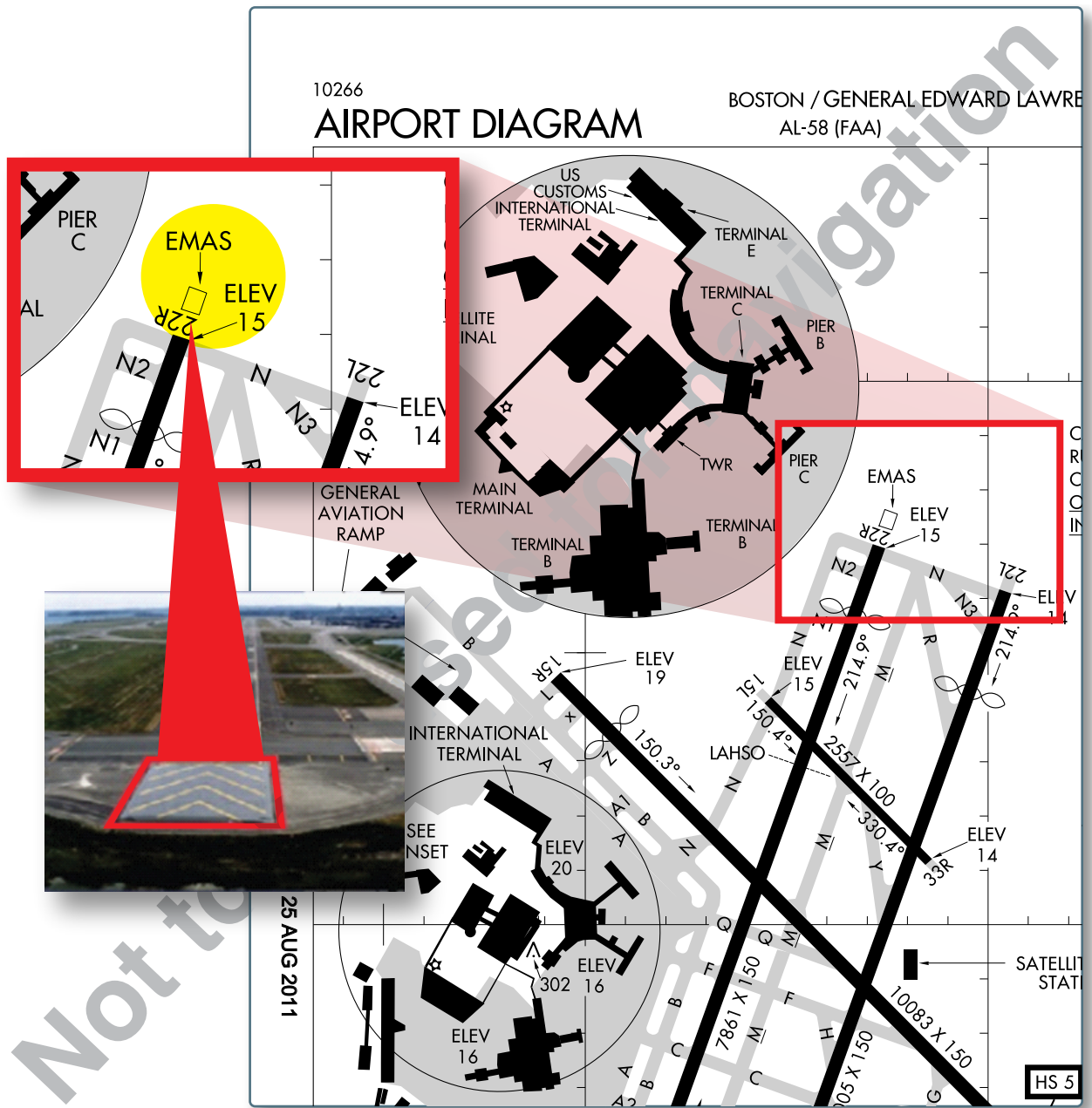
Figure 14-60. An airport diagram with EMAS information.
