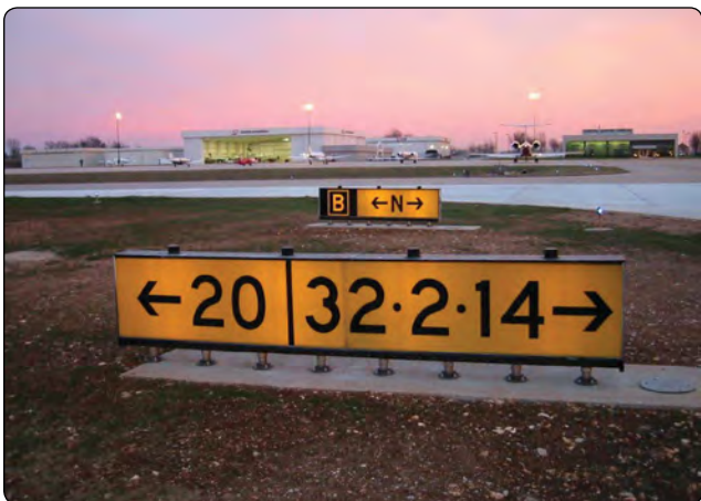
Figure 14-23. Runway destination sign with different taxi routes.
