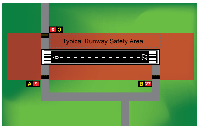
Figure 14-7. Runway Safety Area.
