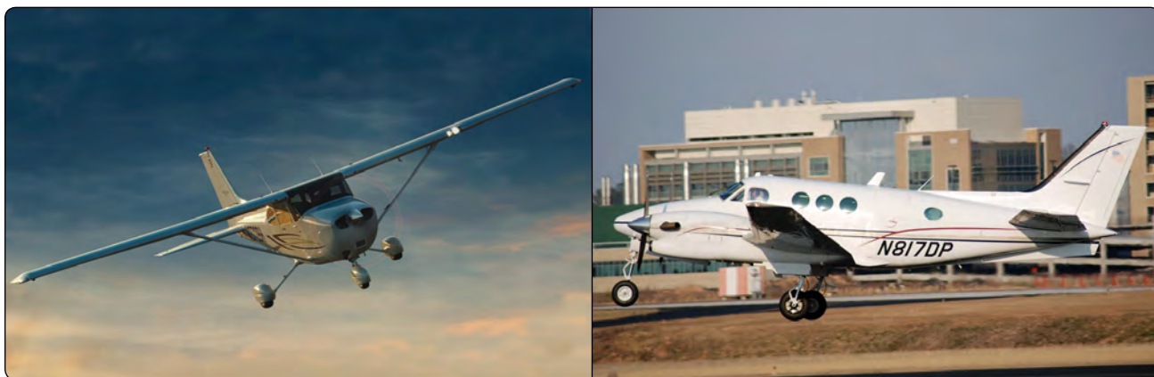
Figure 7-39. Fixed (left) and retractable (right) gear airplanes.
