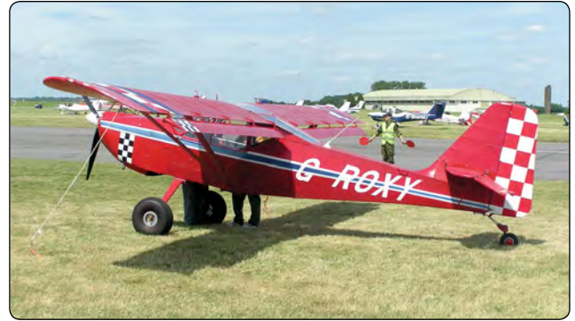
Figure 6-9. Flaperons on a Skystar Kitfox MK 7.
