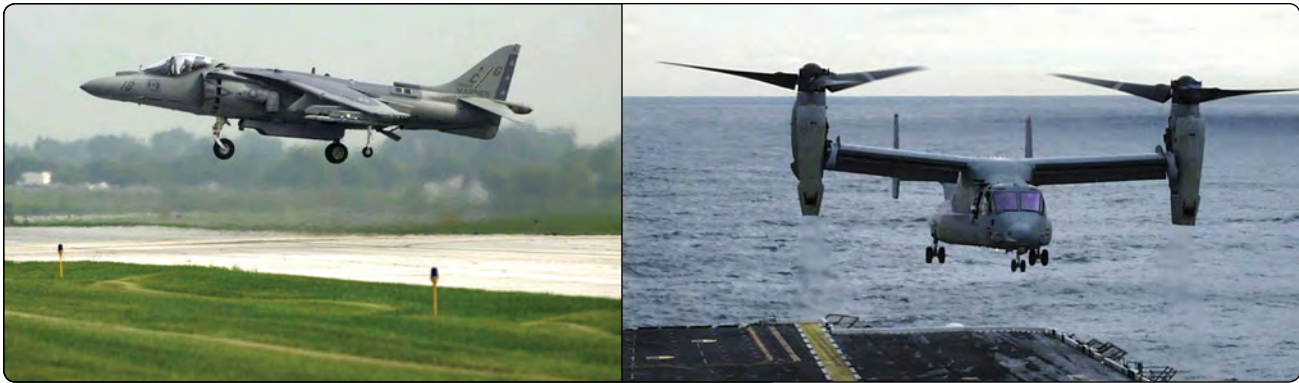
Figure 5-4. Some aircraft have the ability to change the direction of thrust.
