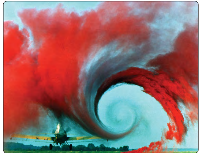
Figure 5-9. Wingtip vortex from a crop duster.
