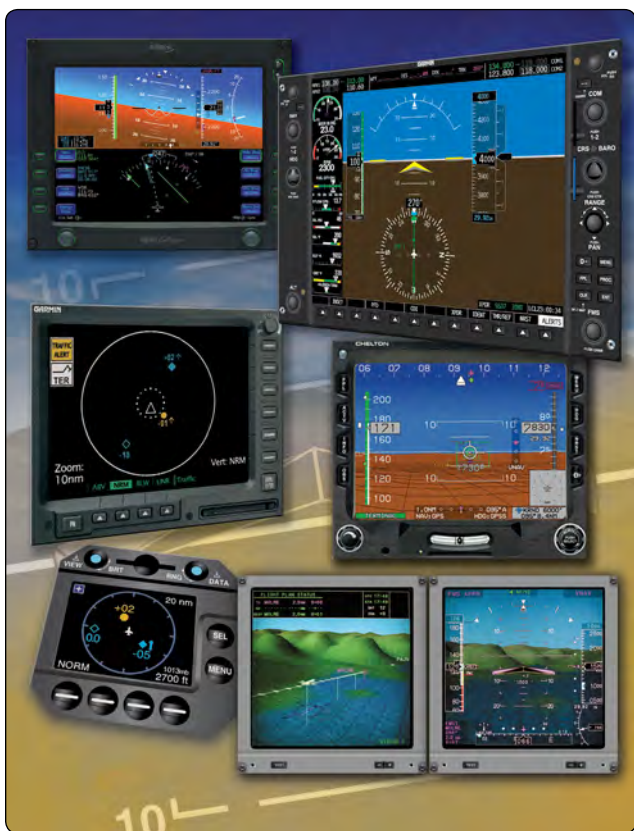
Figure 2-21. Electronic flight instrumentation comes in many systems and provides a myriad of information to the pilot.
