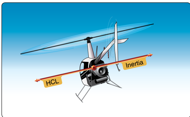
Figure 9-2. During a level, coordinated turn, the rate of turn is commensurate with the angle of bank used, and inertia and horizontal component of lift (HCL) are equal.
