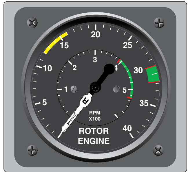
Figure 5-3. Markings on a typical dual-needle tachometer in a reciprocating-engine helicopter. The outer band shows the limits of the superimposed needles when the engine is turning the rotor. The inner band indicates the power-off limits.
