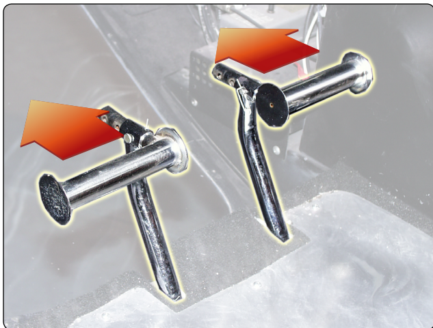
Figure 3-5. Antitorque pedals compensate for changes in torque and control heading in a hover.
