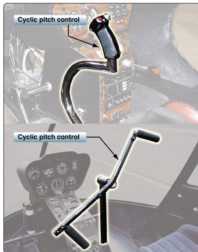
Figure 3-4. The cyclic pitch control may be mounted vertically between the pilot’s knees or on a teetering bar from a single cyclic located in the center of the helicopter. The cyclic can pivot in all directions.
