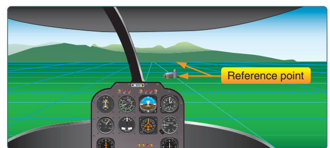
Figure 9-2. To maintain a straight ground track, use two reference points in line and at some distance in front of the helicopter.
