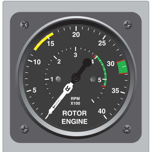
Figure 5-3. Markings on a typical dual-needle tachometer in a reciprocating-engine helicopter. The outer band shows the limits of the superimposed needles when the engine is turning the rotor. The inner band indicates the power-off limits.
