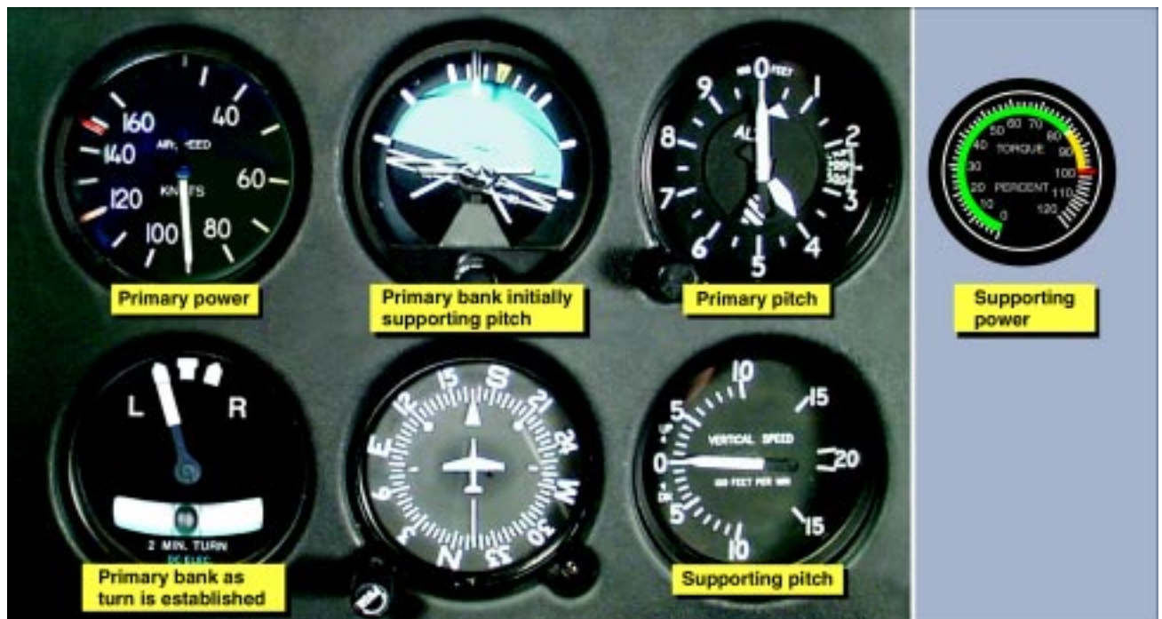
Figure 6-11. Flight instrument indications for a standard-rate turn to the left.
