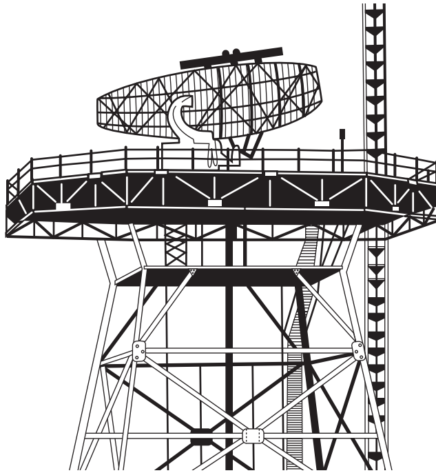
Figure 9-7. Combined radar and beacon antenna.
