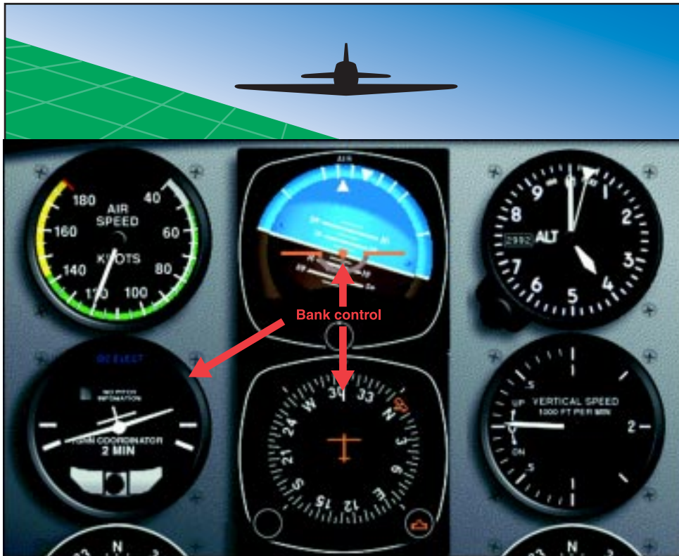
Figure 5-16. Instruments used for bank control.
