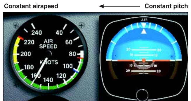
Figure 5-13. Constant power plus constant pitch equals constant airspeed.
