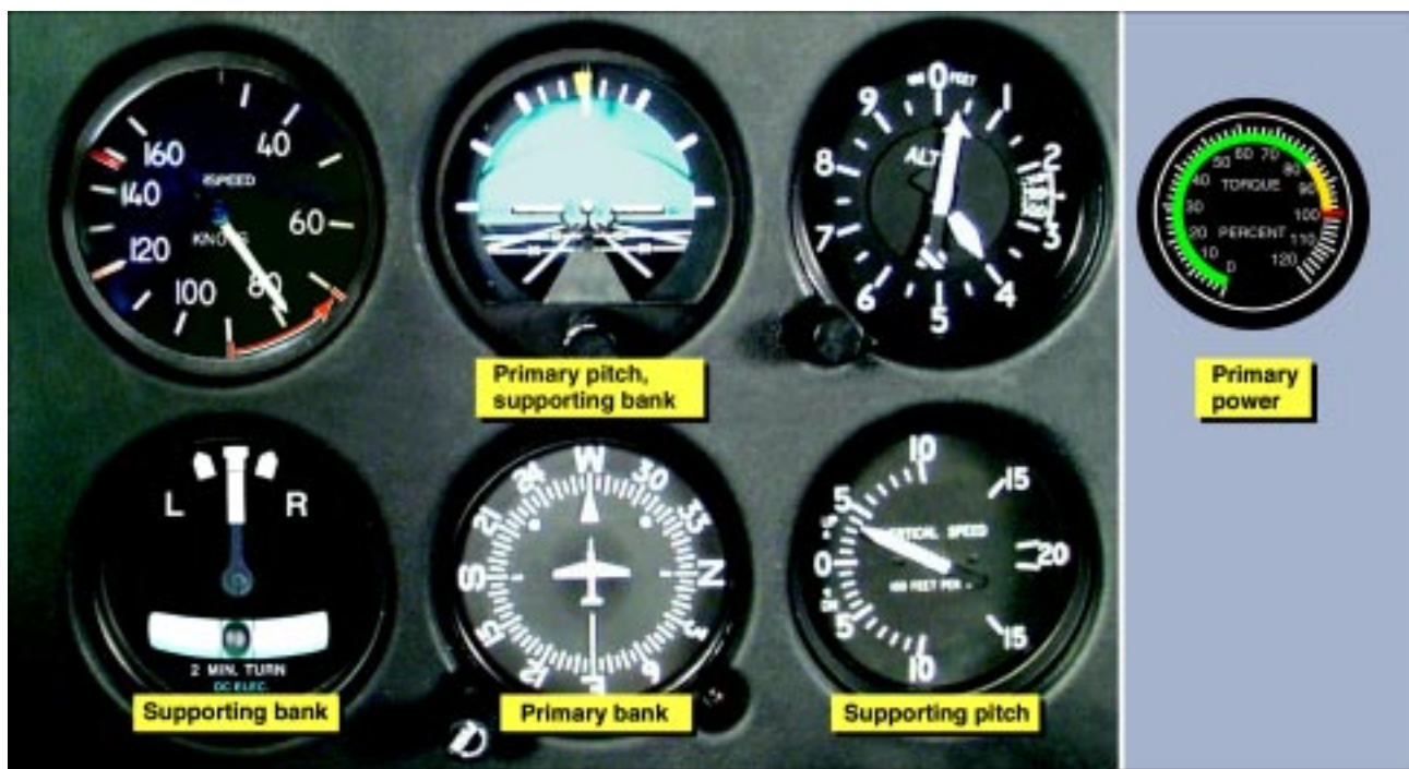
Figure 6-8. Flight instrument indications during climb entry for a constant-airspeed climb.
