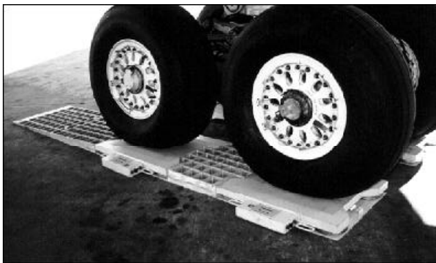
Figure 3-2. Weighing platforms accurately measure the weight of large aircraft without having to raise the aircraft off the ground. (Photo courtesy General Electrodynamics Corp.)
