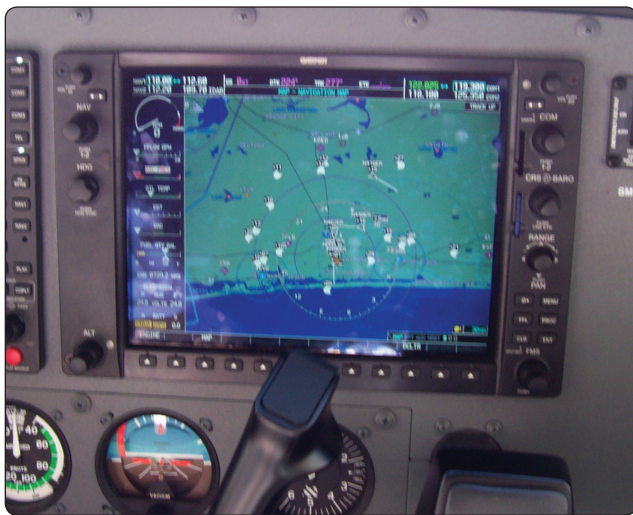
Figure 5-3. Automatic Dependent Surveillance-Broadcast (ADS-B) systems.
